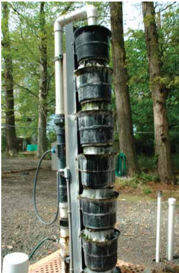
Stony Creek Anglers Club degasses the water using a series of buckets filled with rings to make nitrogen and oxygen levels favorable.
